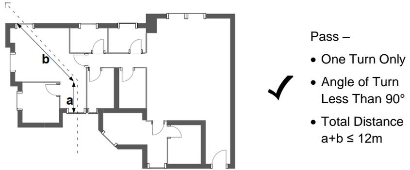
Figure 3 Cross Ventilation Path for Each Habitable Area
