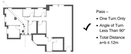
Figure 3 Cross Ventilation Path for Each Habitable Area
