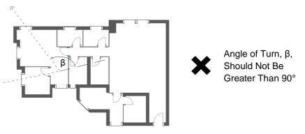
Figure 2 Angle of Turn for the Cross Ventilation Path at the Joint of the Two Lines
