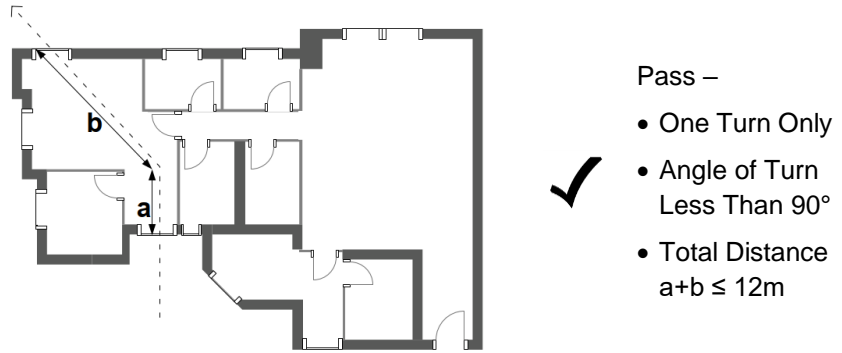
Figure 3 Cross Ventilation Path for Each Habitable Area
