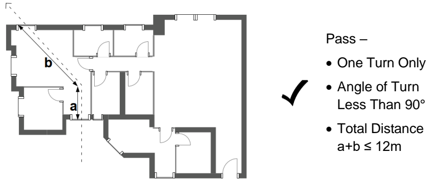
Figure 3 Cross Ventilation Path for Each Habitable Area
